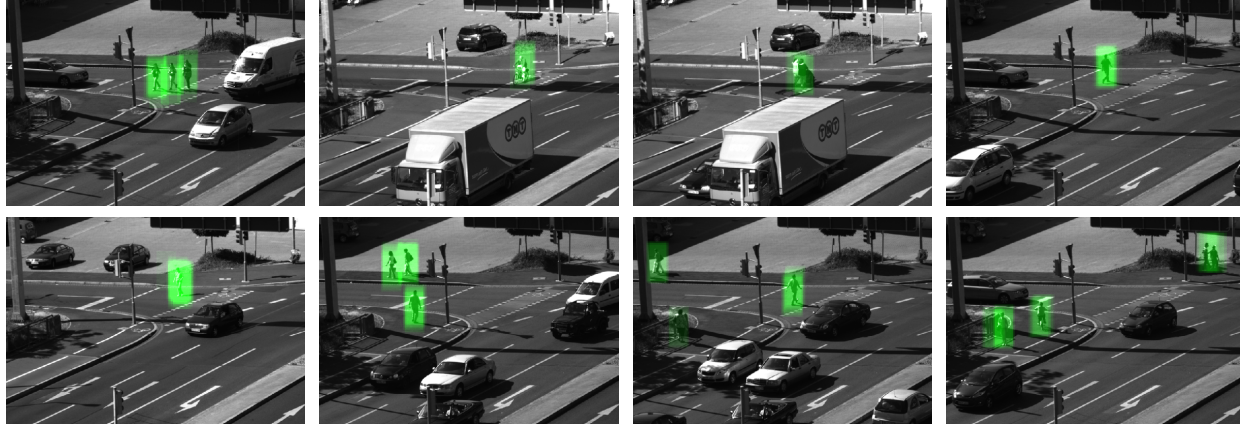
Figure 6. Pedestrian detection results of the HOG-based hypothesis verification from different sequences. Note the detected bicyclist in the first image row, second from left.
