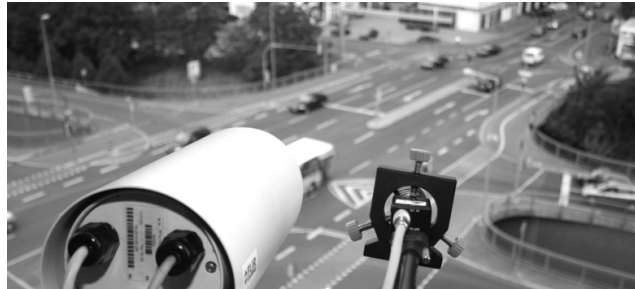
Figure 5. Experimental setup of the road side unit used for evaluation. In the background: target intersection.
