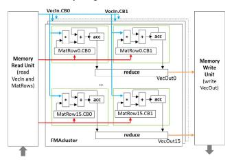
Fig. 3. Accelerator Design. The matrix is divided into column blocks (e.g., CB0, CB1). Each floating-point multiply-accumulate (FMA, in green box) processes a row in a column block, by multiplying input vector (VecIn) elements against matrix row elements (MatRow) kept in on-chip RAMs. Input/output vectors are read/written by memory read/write units.
