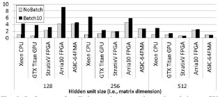
Fig. 5. Performance for all the accelerators under study, relative to CPU performance with no batching.
