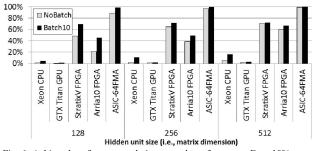
Fig. 6. Achieved performance relative to peak performance. E.g., 10% means the system is underutilized, where the achieved GFLOP/s is only at 10% of the available peak GFLOP/s. On the other hand, 100% means full utilization.
