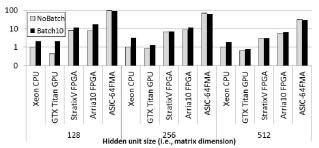
Fig. 7. Performance/Watt for all the accelerators under study, relative to the CPU performance with no batching. The y-axis is in log-scale.
