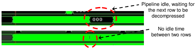
Figure 5-3 Effect of prefetching on pipeline utilization
