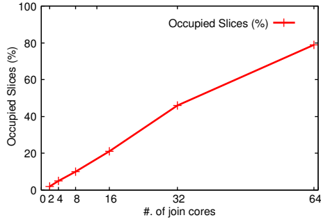
Fig. 11. Overall slice usage of the implemented circuit on a Virtex-6 XC6VLX240T-1 for each of the six different configurations.
