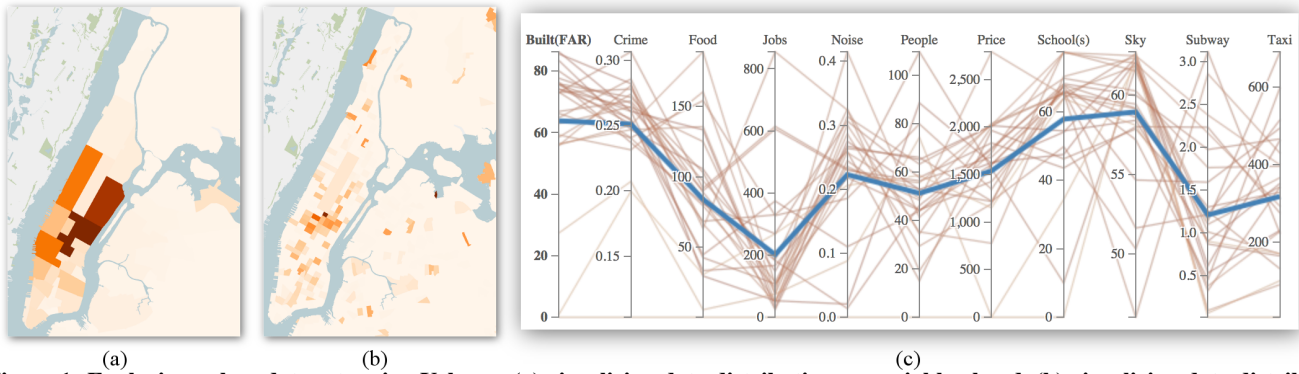
Figure 1: Exploring urban data sets using Urbane: (a) visualizing data distribution per neighborhood, (b) visualizing data distribution per census tract, (c) comparing data over different neighborhoods. The blue line denotes the NYC average for these data.
